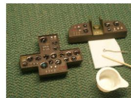
**Final assembly.** To bond the crew and panels in place I use a sharpened wire to poke holes in the balsa cockpit floor. This insures a good surface for the epoxy to attach to. Trace the pilots position with a pencil and make the holes. Apply epoxy to the inside
