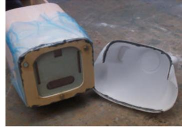
Your cowl might have a small wrinkle Just aft of the scoop. This is the cost of having a one piece cowl and can’t be helped. After the cowl is removed apply epoxy to the inside to form a fillet between the ring and the cowl, this will secure the plastic so you can trim the flange and sand the wrinkle away
