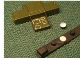
The forward panel has two moon shaped parts that attach to the center of the panel. This is the cradle for the scope tube during takeoff and landing. I have placed mine in the flight mode. Epoxy holds the aluminum tube in place Note the holes drilled in the mount bump
