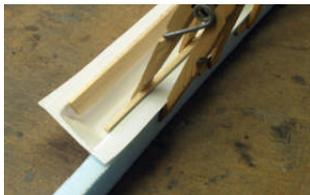
strips as a spacer very useful while clamping the balsa strips to the inside. Allow the strips to overhang the edge then sand them flush. The bond area has a contour. Before you install the fairing cut a hole in the fuselage skin to allow cooling air to pass out the back of the fairing.
