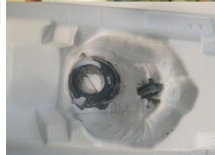
Rough sand the backside of the instrument glare shield to prepare it for the "attachment stick" that engages the fuselage. Apply epoxy thickened with micro balloons ( baking soda works too) to the stick and the cockpit tub. Insert the stick into the hole in the fuselage and seat the cockpit tub in place on the fuselage. Flip the assembly upside-down and make sure the bond is being made by peeking through the forward wheel well.
