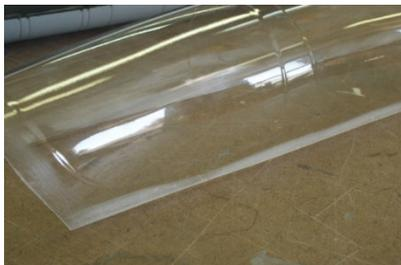
Trim the canopy along the molded lines and check it's fit to the tub with the tub installed on the model. Sand the inside of the canopy edge avoiding the window areas. Clean the canopy one last time and check the cockpit for any details you may have forgotten.
