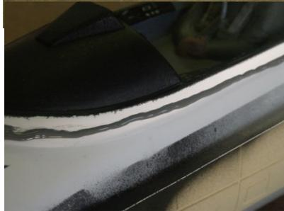
Apply epoxy to the cockpit tub and place the canopy on the tub. Practicing this step a few times before actually doing it will help to get it right the first time. Cutting the corner of a sandwich bag makes a handy way to mix and apply the epoxy.
