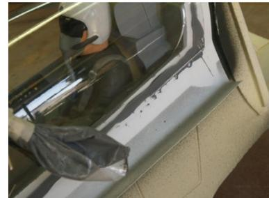
Tape off the windows on the canopy then trim the portion of the cockpit tub used as an "epoxy bib". eave about 1/8 inch of the tub around the edge to leave a thin looking panel line. Prime and paint. if you can't find the perfect color match for your model foam safe paint will allow you to overlap colors like the green below making the mismatch is less noticeable. The tan color used below is not foam safe paint and must be applied to the canopy only.
