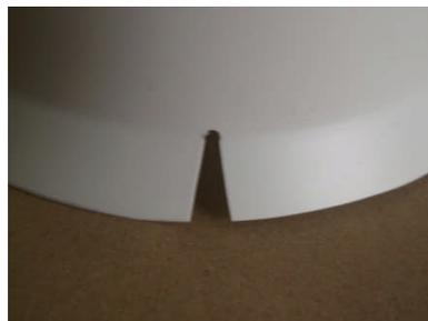
copied properly. Drilling the holes is a preventive measure meant to avoid possible cracks in your cowl. Using scissors is easy but sets up a shear pressure at the gap. The drilled hole simply relieves the pressure.
