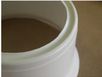
There is a groove molded into the top of the base. This groove should be retained if possible, it acts as a former and stiffens the mid section of the cowl. Test fit the assembled cowl to the model, you may want to adjust the length.
