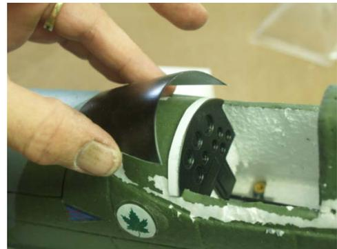
Note a bit of the glare shield edge will need to be trimmed to prevent the canopy from being raised from the model when it is bonded in place. Test fit the seat back and trim away plastic or foam preventing it from seating completely.
