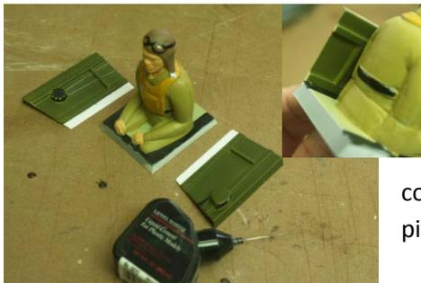
Bond the cockpit sides in place with the slanted end at the front and the aft end flush with the aft corners of the cockpit bottom. After the glue sets, test fit the pilot assembly. The upper lip of the cockpit sides are wider than the foam edge and will require trimming. Practice the installation of the cockpit up grade before applying epoxy. I found that installing the pilot in place first then sliding the ends in the gaps worked best.
