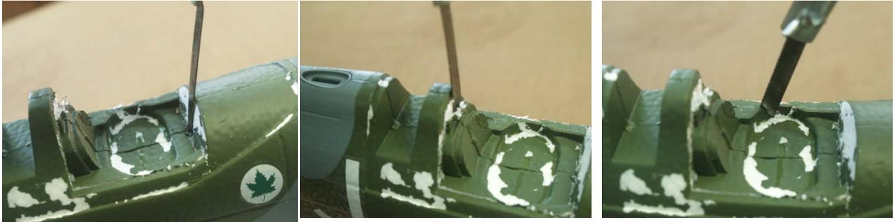
Remove the foam and clean up any gaged edges with the knife. while you are there use epoxy to lock down the pushrod tubes for a more positive feel to the controls . If you test them you will see they have some play.
