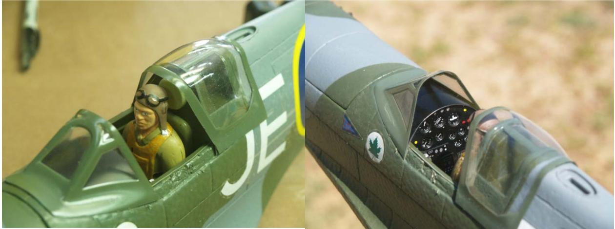
You might consider carefully cutting the canopy and flying with an open cockpit to show off your details. The plastic is thick enough to put up with the wind and I have not noticed any difference in flight performance.
