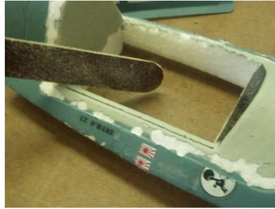
To start the upgrade carefully remove the stock canopy, to avoid lifting the paint lightly (shallow) cut around the canopy. Cut the bottom of the canopy away at a 90 degree angle then make a mark 1/8 inch from the outer edge of the cockpit sides.
