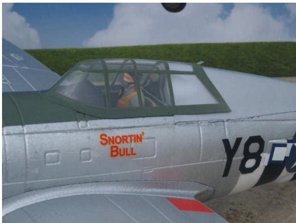
To hold the hatch closed, cut holes in the fuselage about even with the pilot. Bond magnets in the fuselage first using a flat piece of metal to hold it flush while the epoxy sets up.
