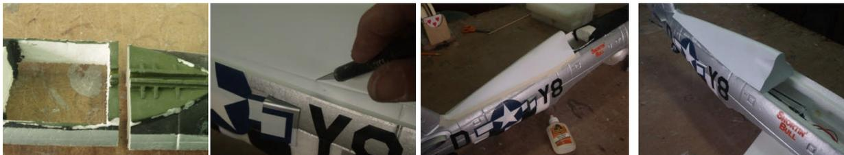
if desired. Rough sand the two surfaces and use Gorilla glue or silicone to attach the turtle deck. Complete the cockpit detail as described above.
