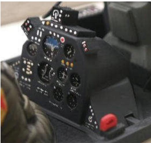
The instrument panels are fairly straightforward. Scuff up the bottoms so the epoxy will hold better. Just a few tips: Spray paint them black then use something sharp to scratch the dial markings on the instruments. Apply a drop of epoxy in the instrument holes to simulate glass. Add a little paint and you are done.
