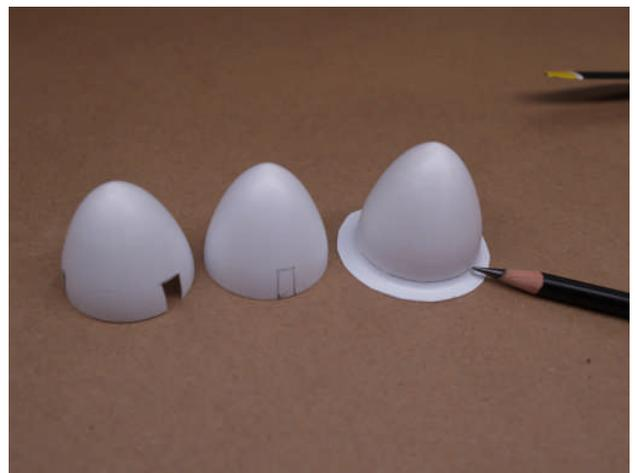
Depending which motor assembly and prop you use will change how the spinner will be installed. The faint marks on the spinner are for a two blade propellers. For three blade props, you will need to carefully mark where the spinner will be trimmed. Use a pencil laying flat on the work surface and mark a trim line then cut. Center the spinner on the prop and make the marks where they contact the spinner and cut the slots.
