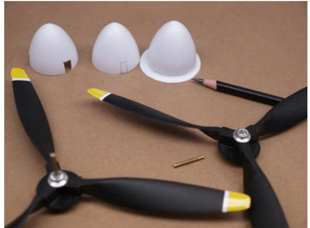
dries. (Give it a whole day. For prop adapters that have no shaft, an extension can be made by drilling a small hole and bonding a brass pin in place.
