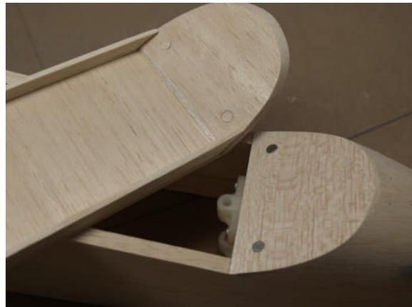
Paint the cockpit floor black then use a pencil to mark the locations of the crew, seats and panels. Use a sharp object to puncher the balsa on the inside of the pencil line. I used a throwing dart. This will help make a better bond. After the canopy is in place, there is no access to the crew. Apply epoxy then bond them in place.
