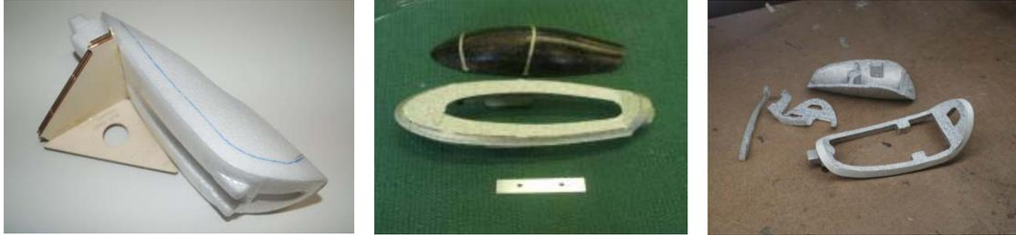
adhesive will work but can cause a haze around the window as it dries. Canopy glue can be used however silicone adhesive has worked best.
