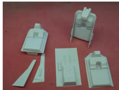
One half has a bond step while the other has a trim line formed in it. Trim to the line and on the other, trim to get the widest bond but remove the portion of the plastic did not touch the form tool. (Remove the roll for a flat surface) At the front, trim 1/2 inch from the step. This lip is needed to attach the cowl, save the scrap. Where the nacelle meets the wing, leave your self about 1/2 inch to make a bond.
