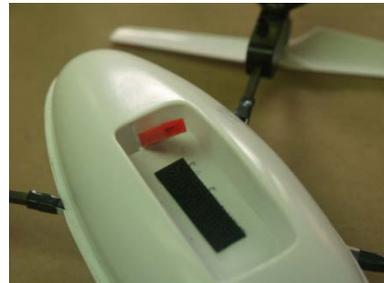
To keep the battery lead from entering the Pod cut a square hole and a slot for the wire in the front end. To install the battery ;attach it to the connector and feed it through the square hole and hold it in place with Velcro. When the battery is not in the compartment the wire is slid into the slot to prevent it from entering the pod.
