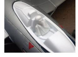
The halves bond with model cement then painted. There is a groove formed in the tub so improper placement would be very hard. After the painting is complete bond the pilot into the groove and trim the canopy along the bottom edge. sand the bonding surfaces and apply epoxy to attach the
