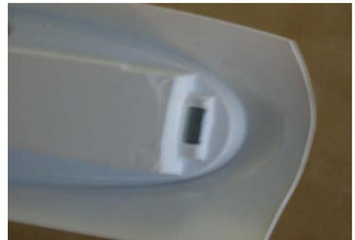
hold down the plastic wrap. Apply a dab of epoxy to the magnet and the space in the tub and install the tub in the fuselage with a weight to hold it down. I like JB weld due to its viscosity, however baking soda can be added to epoxy to make it thicker. The point is you don't want to allow it to be running all over and making a mess of things.
