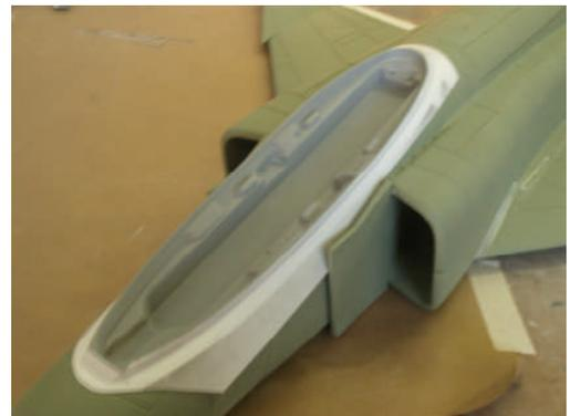
I used cement to bond the forward panel and glare shield in place and switched to silicone as a bonding medium for the rest because it allows adjusting time. As each part goes in place, test the canopy fit to ensure the crew and seats don't interfere with the canopy fit.
