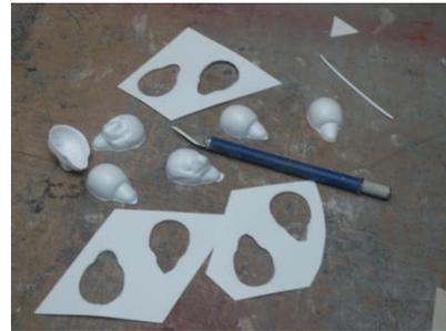
cement to bond the halves together. Keep a rag handy to keep your fingers clean. A piece of folded masking tape applied to the front of the parts is a handy way to attach a handle to the parts for easier manipulation.. Model cement is a solvent based adhesive and does not sand well until it is completely dry. So, allow the heads to dry overnight. Sand the seam and prime the head. Check the pilot painting instructions on the website for the rest.
