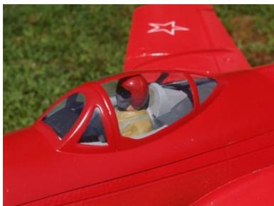
This upgrade kit was designed to be independent from the stock hatch so you could have a spare for whatever reason. The stock hatch can be used if desired. To install, cut the foam away horizontally just under the window line and a little vertically around the tub area. The tub and canopy should be bonded to the hatch while installed on the model to prevent changing the shape of the foam hatch.
