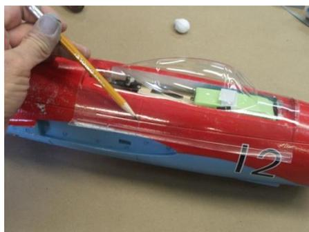
Align the canopy over the fuselage matching the molded panel lines with the lines formed in the canopy. Mark and trim the ends keeping as much overlap as possible end to end. the amount of plastic used from side to side is up to you.
