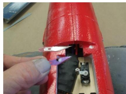
After the epoxy sets up remove the blades and cover the magnet areas with plastic sandwich wrap. allowing the second magnet to hold it in place. Place the canopy back on the fuselage and mark the spaces over the magnets. sand the inside of the canopy around the marks for a good bond.
