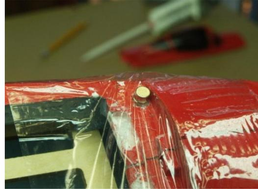
Apply JB weld epoxy or thickened hobby epoxy over the magnets and place the canopy in position. turn the model upside down to allow the epoxy to contact the canopy surface. note you should practice this step and if tape is used to hold the canopy in position use "low stick" or painters tape to prevent removing the paint from the fuselage when peeled off.
