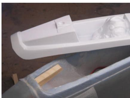
While all that is drying ,trim the cockpit tub along the trim line ( molded in the tub) Line the fuselage with sandwich plastic wrap to protect the foam and install the provided stick. Sand the inside of the cockpit tub at the glare shield for a good bond,
