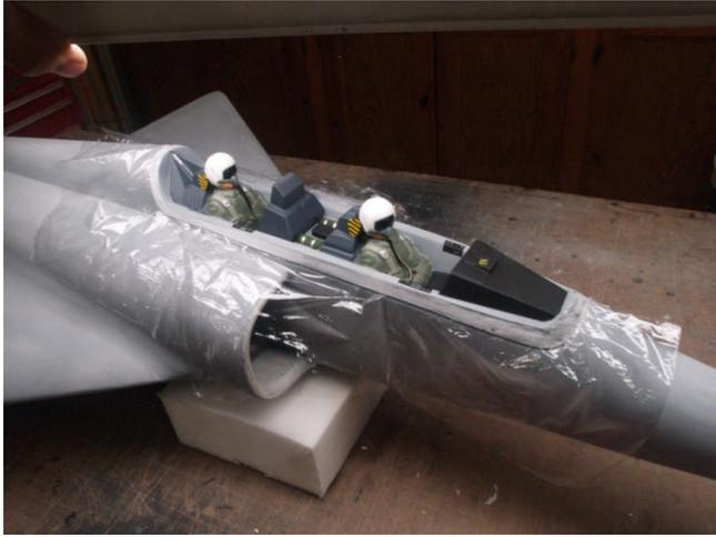
Rough sand the bond joint area between the canopy and cockpit tub to ensure a good joint. Line the fuselage with sandwich wrap to protect the foam like you did before , install the cockpit Tub and rough trim the canopy so it will fit over the assembly. Use a sharpie marker to mark the canopy trim line starting at the top front and back. This will
