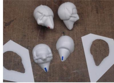
Apply model cement to the edge of one of the halves and align them where the neck meets the helmet. Allow the head to dry overnight before trying to smooth the seam.
