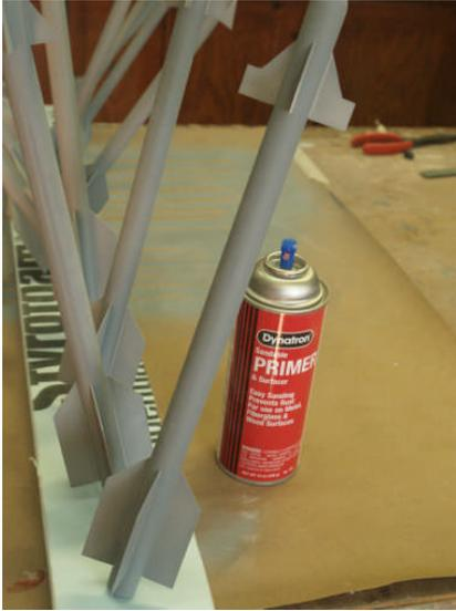
Nails pushed into a foam board makes a nice drying rack but when you paint the missile it is much easier to have a long dowel handy to use as a handle. The dowel can be rotated to spray an even coat and if it's long enough it can be placed on a table with the missile hanging over the edge to dry.
