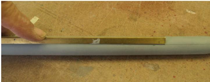
Use a piece of angled stock to draw the lines for the fins using the marks. Anything with a parallel 90 degree straight edge will do, example: a tool box drawer handle or the guide groove in a table saw top.
