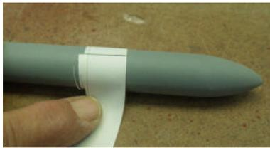
Wrap a piece of paper around the missile body and make a mark where they overlap.
