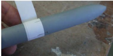
Fold the paper into quarters and mark the folds. Wrap the missile with the paper once more and align the marks so they miss the body seams.
