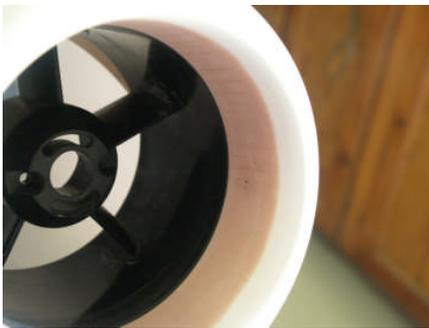
together leaving one seam not bonded. Insert the cowl halves into the inlet ring and expand the cowl until it fits tight. Apply tape to the cowl / ring seam. Mark the cowl piece without the formed step so the trim line matches the step in the opposite side. Apply adhesive to the seam with the inlet ring in place. For better fan performance, a thin layer of automotive body filler can be applied to the ring to smooth airflow. Bond the cowl to the inlet
