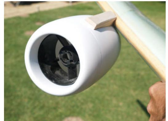
ring and allow it to dry overnight. To install the cowl to the model the fan unit should be removed until the cowl has been trimmed to fit the motor pylon. (Cutting out one of the cowl seams while fitting makes a neater cowl.) The cowl is attached to the pylon with silicone so it may be removed, the inlet ring is held in place with a tight fit only.
