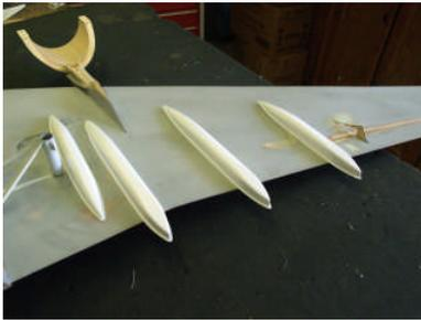
The dummy flap hinge fairings trimmed leaving a 1/8 inch flange around its base. Epoxy is used to bond them to the wing. The engine cowl comes in three pieces. The inlet ring is marked with a pencil laying flat on the table and cut with
