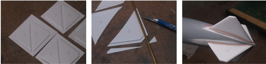
the fins together using the edges for alignment. Allow the fins to dry overnight. Rough cut the flange with scissors and then block sand the flange to 1/32 inch from the fin edge. Apply a small amount of filler to the edges to hide the bonding flange then block sand the fin edges to shape.
