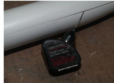
The remaining half is used as a doubler, cut it in half to form two strips and bond it to the inside of one of the tank halves.
