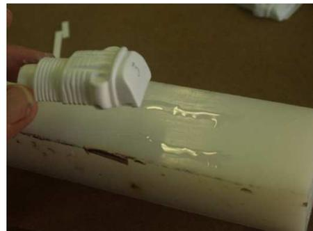
After the paint is applied ( most spray paints are compatible) scratch the surface of the cylinder heads to remove the paint where they will touch. Use the engine case to as a fixture to align the heads and bond them where they touch. A straight edge along the cylinder parting seam will ensure they are aligned.
