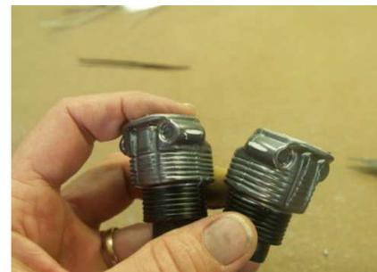
scratch the paint off the engine case where the cylinders will bottom out. and bond the cylinder pairs in place. Be sure to look at the front of the motor straight on to make sure they are not drooping down.
