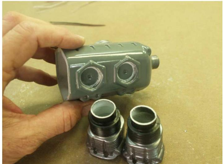
drill holes for the push rod tubes and slide them in place, coffee straws or aluminum tubes work well for this, secure them with a dab of epoxy or silicone before bonding the valve covers in place.
