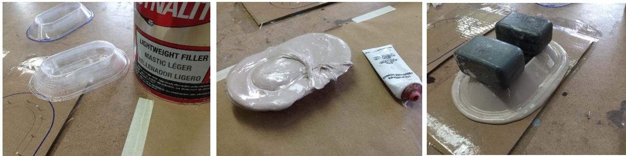
Mix the filler and fill the inside of the chock with a little mound in the middle. Quickly place the chock on the cardboard over the nails and press down to squeeze out some of the extra filler. When the chock becomes warmer than room temperature the filler is firm enough to trim with a hobby knife.
