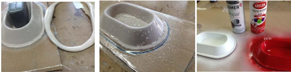
After you trim the excess away monitor the chock temperature; the filler can get hot enough to distort the plastic. Just keep it wet and it will do fine. Remove the chock from the cardboard, sand the edges to your liking and give it a coat of paint. I suggest a bright color so they are not left at the flying field.
