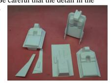
One half has a bond step while the other has a trim line formed in it. Trim to the line and on the other, trim to get the widest bond but remove the portion of the plastic did not touch the form tool. (Remove the roll for a flat surface) At the front, trim ½ inch from the step. This lip is needed to attach the cowl, save the scrap. Where the nacelle meets the wing, leave your self about ½ inch to make a bond.
