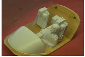
**Seats** Bond the front and back halves together. Be careful that the detail in the backside is not part of the bond. Use scrap plastic to bond a plate to the inside of the seat side. Bond the seat sides to the seat then allow it to dry over night. Sand or trim the excess plastic away from the seat. Bond to cockpit with silicone.
